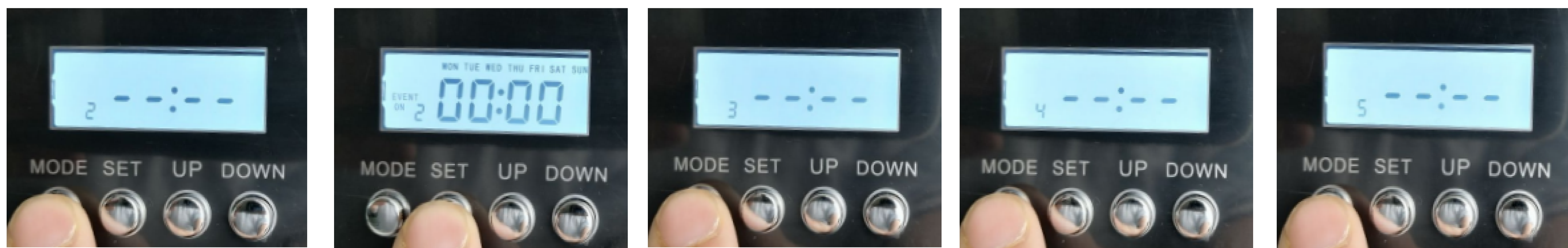
3.1 Press "MODE" till above page show. if you want set up other work interval, you can press "SET" button to adjust, same operation (2.1--2.10) in step 2
