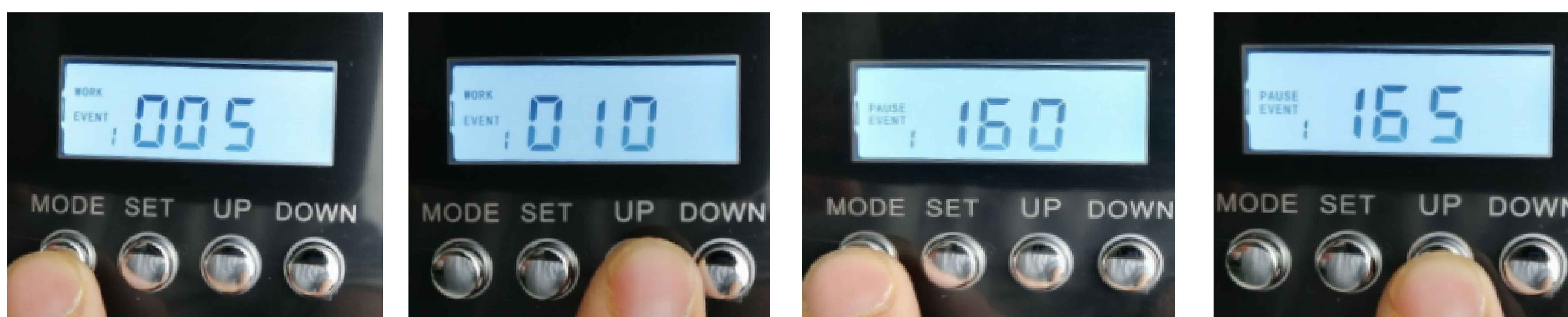
2.9: Press "MODE" till above above page show "WORK EVENT 1", then press "UP" to adjust
