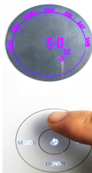
Step 12: press UP button, adjust into 5ml/h. then click SET button again to save setting
