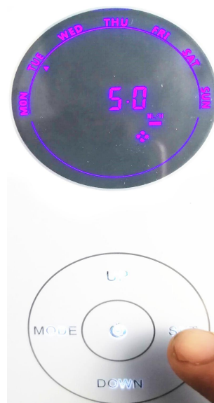
Step 11: press SET button till oil consumption page show. Fixed is 5ml/h
