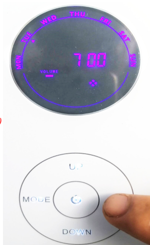
Step 7: press SET button till above page show, this is bottle volume. Fixed Volume is 2000.
