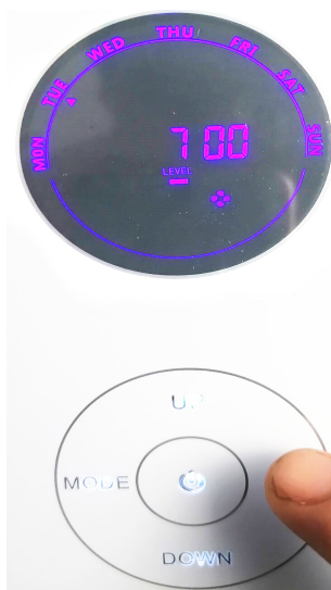
Step 9: Press SET button till oil volume page show. it is oil volume in bottle. If have 800ml oil in bottle
